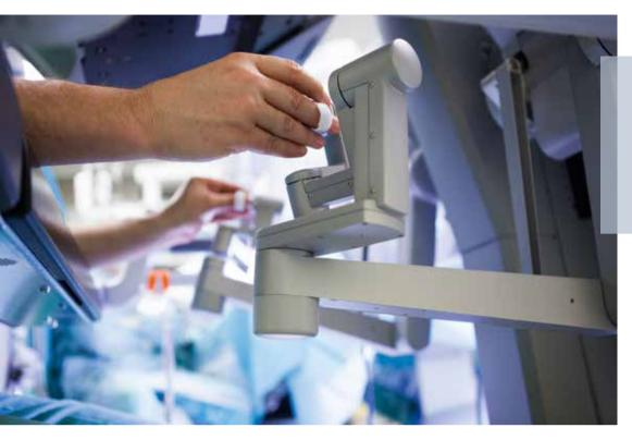
With the Da Vinci operation system, the operator can control the arms and instruments of the robot with millimetre precision using his hands.
